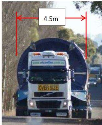
Figure 1 – Approximate maximum required trailer width and height dimensions (depending on turbine model and trailer type)
